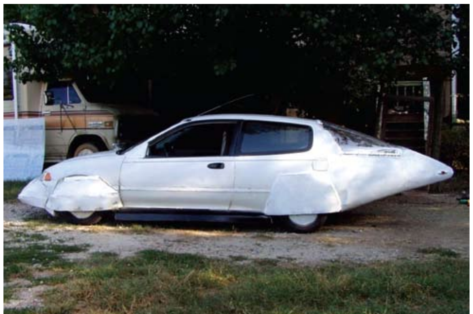
The owner of this 18-year-old Honda Civic modified it with handtools to raise it from 80km/4.5l to 150km/4.5l.
